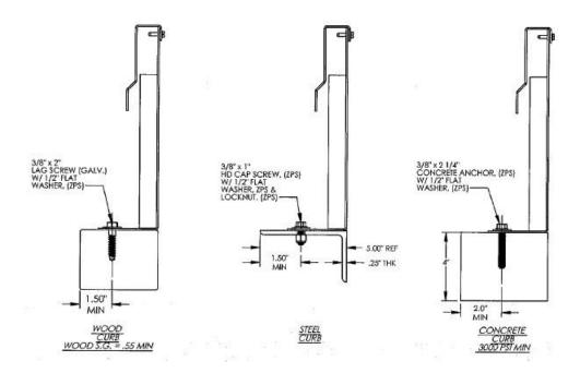
Mark the pre-drilled 3/16 inch diameter holes from the mounting flange through to the roof deck, typically into a built-up wood fame curb. Fasten roof hatch curb flange to framing using roofing nailers and/or screws, recommended size 3/16 inch by 1-1/4 inch long.
