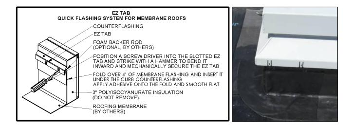
Install roofing material up to and around the roof curb, up under the counterflashing, using appropriate roofing material and locally accepted processes. Do not remove curb insulation. Lay membrane flashing up onto curb insulation. Press up under counterflashing using foam backer rod (by others). Apply adhesive to fully secure membrane in position. Ensure all joints are fully sealed to provide a weather tight seal. Bend EZ tabs to mechanically secure, using a screwdriver or similar tool.
