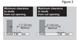
4. Cut the opening with a knife, saw or drywall cutter. Make sure the edges are clean.
