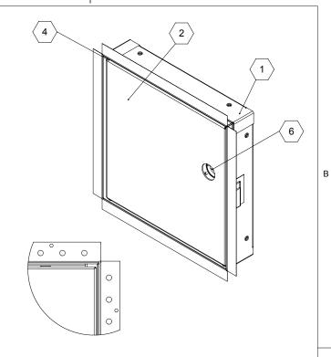
DETAIL D DRYWALL BEAD DETAIL SCALE 1 : 4
